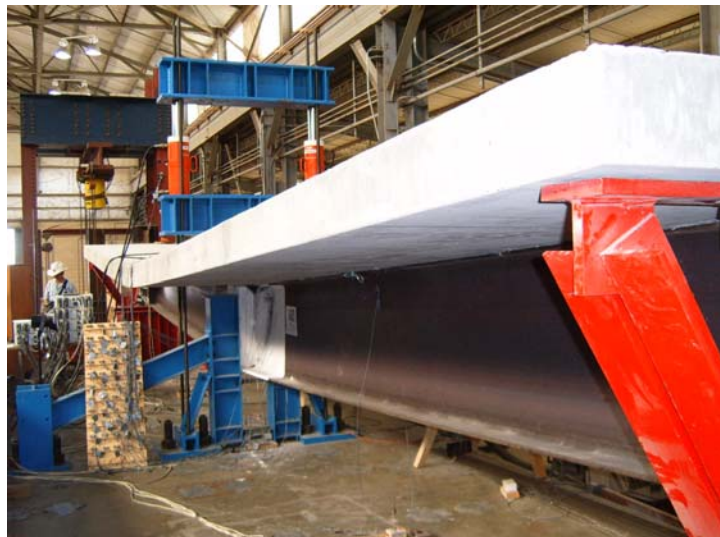
Figure 4.26: Specimen NON-00BS – Overall view of specimen at end of test (11.5-in. deflection)
