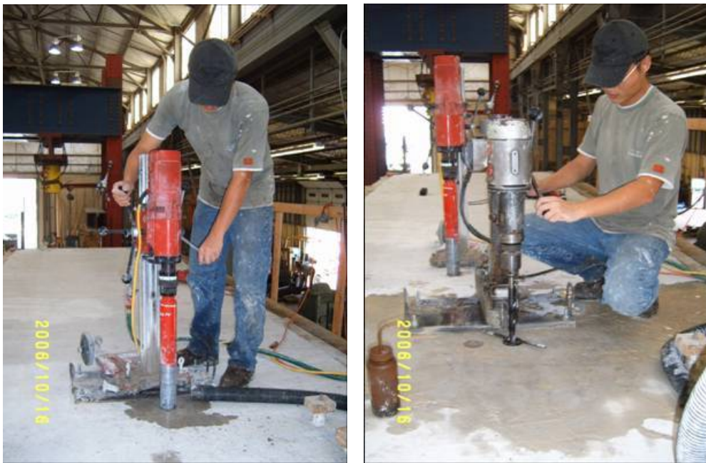
Figure 4.5: Coring and drilling into the specimen
