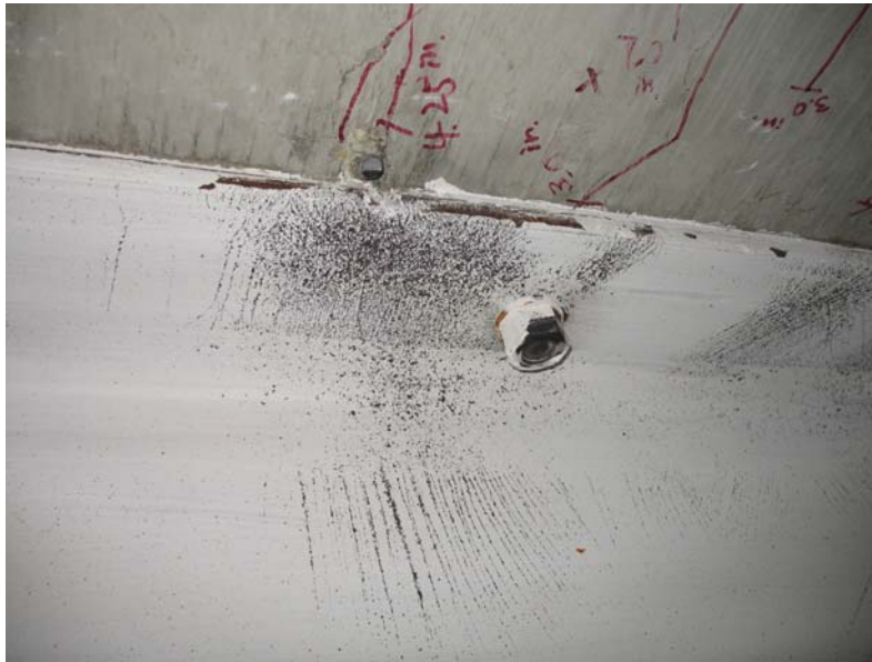
Figure 4.38: Specimen HTFGB-30BS – flange local buckling (11.0-in. deflection)
