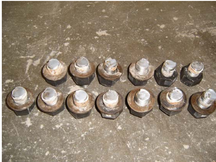
Figure 4.30: Specimen HASAA-30BS - Failed shear connectors
