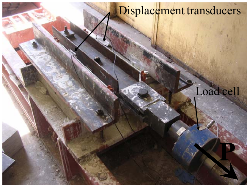
Figure 3.14: Instrumentation for single shear connector tests
