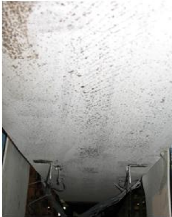
Figure 4.32: Specimen HTFGB-30BS – Whitewash flaking (6.5-in. deflection)
