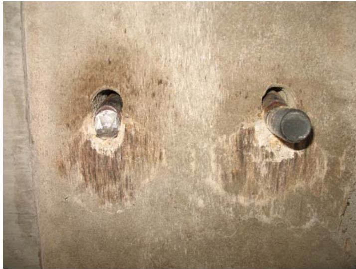
Figure 4.35: Specimen HTFGB-30BS – shear connectors after the test (slab bottom)
